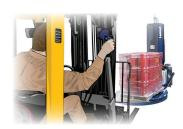
Click-n-Go remote meets the latest safety requirements outlined by the National Electrical Code. Using infrared technology and two-step activation process, the Click-n-Go is immune to accidental activation from stray radio frequency.
