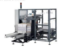
**MultiFormat:** MFC1000/2000 Up to 4 blank magazines with different case sizes. Speed varies.
