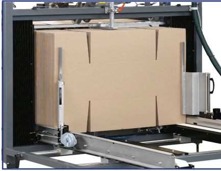
Blank Delivery Control Powered belts precisely govern the delivery speed of the tray blanks. Blank retainers ensure the blanks are spaced correctly.
