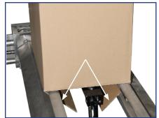
**Stationary Flap Folding** Once the case is square, it remains square by folding the flaps while it's stationary. This makes the case rigid and locks in the 90 degree angles.
