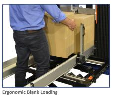
Easy to load magazine. Replenish blanks while machine operates. Simple and fast magazine adjustments.
