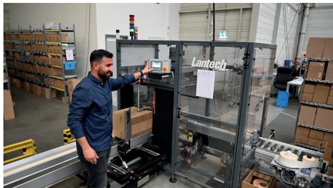
Eurapon's operations manager Yilmaz Akin in front of a C-1000 case erector. The C-1000 combines speed with flexibility. Many types of cases and closures can be processed with this system.
