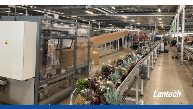
After manual filling with houseplants, the CS-1000 Tape case sealer reliably seals the shipping packaging with adhesive tape. The machine is optimised for the upstream case erector. Bunnik Plants now achieves an output of 13 cases per minute on the packaging line, the operating flow is constant and system stops are very rare. On this line alone, three employees could be saved and made available for other tasks.
